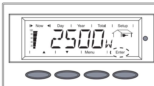
Display mode 'Now', energy currently fed into the grid with 'Enter' key enabled
